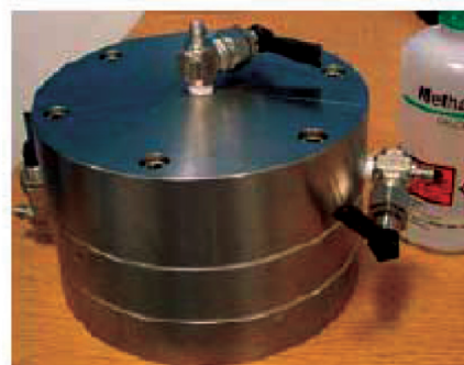
Figure 46. Pressure driven parallel capillary reactor. Reproduced from Beilstein Journal of Organic Chemistry (Styring, P.; Parracho, A. I. R. From discovery to production: scale-out of continuous flow meso reactors. Beilstein J. Org. Chem. 2009, 5, 29; http://www.beilstein-journals.org/bjoc/single/articleFullText.htm?publicId=1860-5397-5-29 ), 172 under the terms of Creative Commons Attribution License ( http://creativecommons.org/licenses/by/2.0 ) and subject to Beilstein Journal of Organic Chemistry terms and conditions ( http://www.beilstein-journals.org/bjoc ). Copyright 2009 Styring and Parracho.
